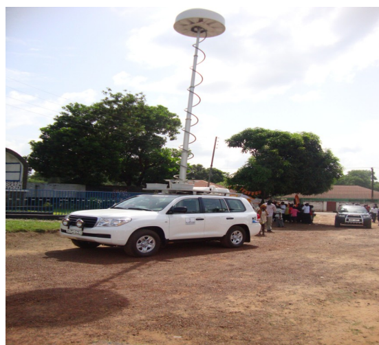
NATCOM Spectrum monitoring equipment mounted on a van in Kenema, Sierra Leone
